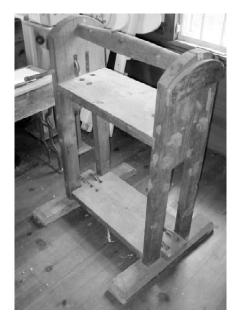
The *whatisit* has a moveable shelf at the bottom that has 2 pulleys at each end of the shelf, with matching pulleys at the top of each side. The windless at the top has holes in it so that short poles can be inserted to wind the bottom up to compress what ever was being compressed.
